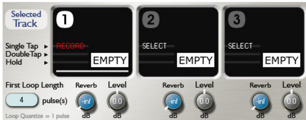
This section shows the three looping tracks with their mix knobs and the loop quantize button.
